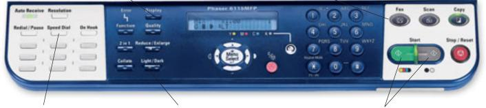
Fax function buttons include one-touch dialing, Speed Dial and Resolution settings.
